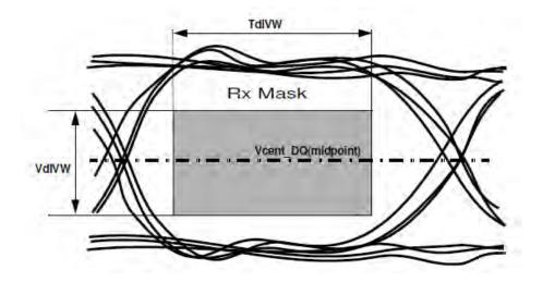
Figure 211 — DQ Receiver(Rx) compliance mask
