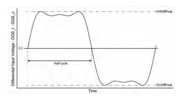
Figure 199 — Definition of differential DQS Signal AC-swing Level
