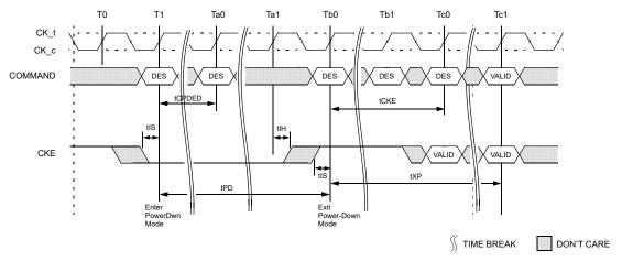
Figure 153 — Precharge Power-Down Entry and Exit
