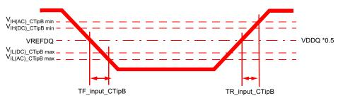
Figure 167 — Input B Slew Rate Definition
