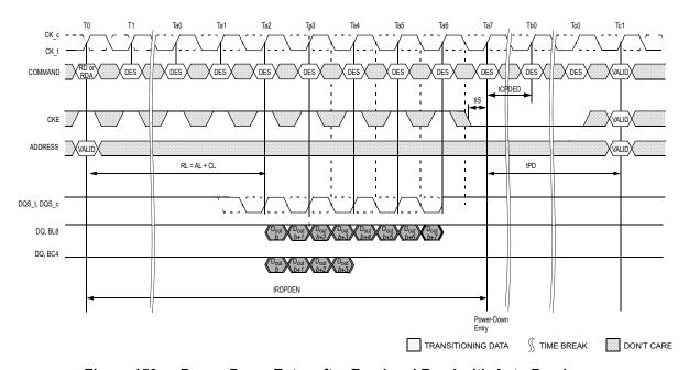
Figure 150 — Power-Down Entry after Read and Read with Auto Precharge
