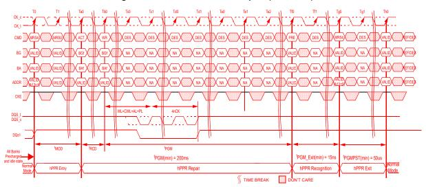
Figure 172 — Hard Fail Row Repair (WR Case)
