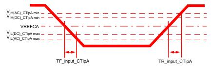
Figure 166 — CS\_n and Input A Slew Rate Definition
