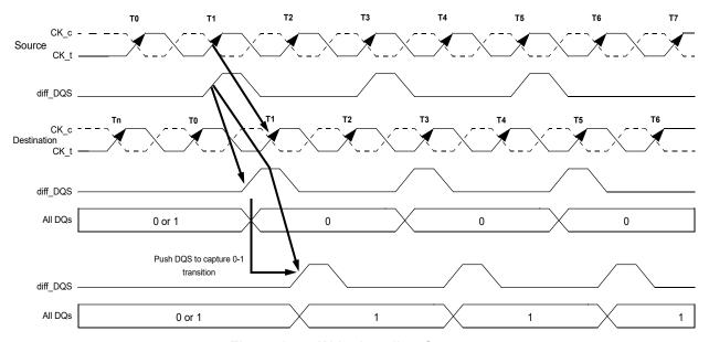
Figure 14 — Write Leveling Concept
