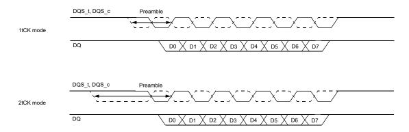
The timing diagrams contained in Figure 66, Figure 67 and Figure 68 illustrate 1 and 2 tCK preamble scenarios for consecutive write commands with tCCD timing of 4, 5 and 6 nCK, respectively. Setting tCCD to 5nCK is not allowed in 2 tCK preamble mode
