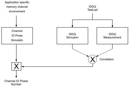
Figure 209 — Correlation from simulated Channel IO Power to actual Channel IO Power supported by IDDQ Measurement
