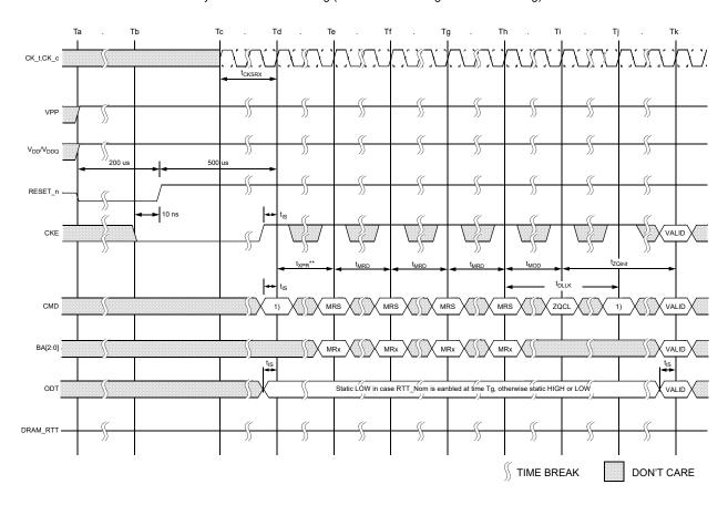
NOTE 1 From time point 'Td' until 'Tk', DES commands must be applied between MRS and ZQCL commands.
