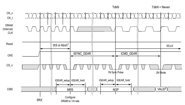
NOTE 1 CKE High Assert to Gear Down Enable Time (tXS, tXS\_Abort) depend on MR setting. A correspondence of tXS/tXS\_Abort and MR Setting is as follows.
