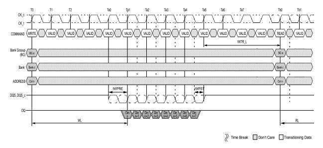
NOTE 1 tWTR\_L: Delay from start of internal write transaction to internal read command to the same Bank Group. When AL is non-zero, the external read command at Tb0 can be pulled in by AL.
