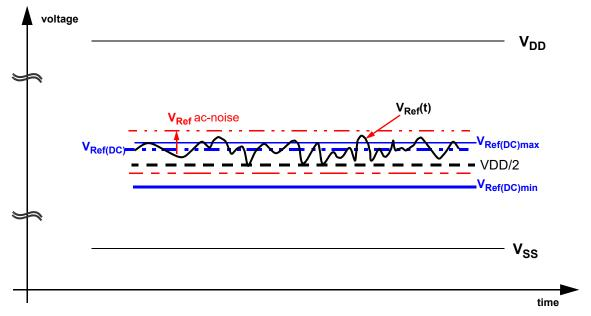
Figure 189 — Illustration of V<sub>REF</sub>(DC) tolerance and V<sub>REF</sub> AC-noise limits
