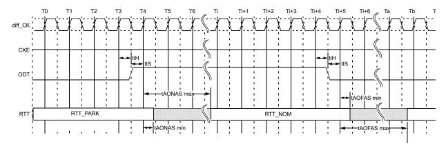
Figure 182 — Asynchronous ODT Timing on DDR4 SDRAM with DLL-off
