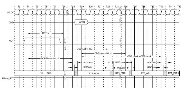
Figure 177 — Synchronous ODT example with BL=4, CWL=9, AL=10, PL=0; DODTLon/off=WL-2=17, ODTcnw=WL-2=17
