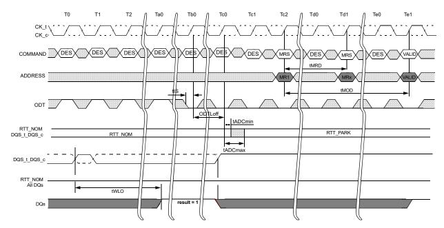
Figure 16 — Timing details of Write leveling exit
