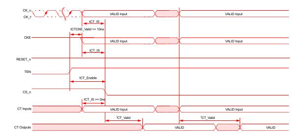
Figure 164 — Timing Diagram for Connectivity Test(CT) Mode
