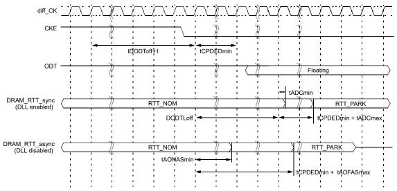
Figure 183 — ODT timing for power down entry with ODT buffer disable mode
