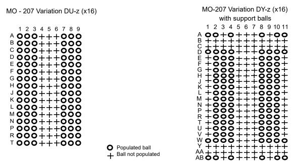
Figure 2 — DDR4 Ball Assignments for the x16 component
