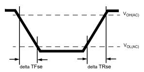
Figure 204 — Single-ended Output Slew Rate Definition
