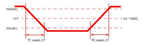
Figure 206 — Output Slew Rate Definition of Connectivity Test Mode
