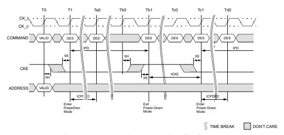
Figure 158 — Power-Down Entry/Exit Clarification
