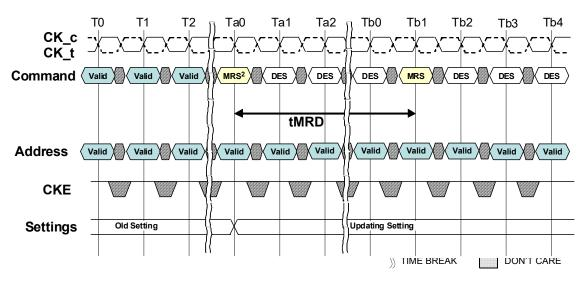
NOTE 1 This timing diagram shows C/A Parity Latency mode is "Disable" case.
