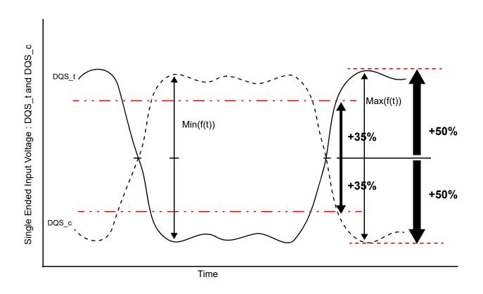
Figure 200 — Definition of differential DQS Peak Voltage and rage of exempt nonmonotonic signaling
