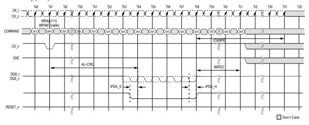
Figure 161 — Maximum Power Saving mode Entry with PDA
