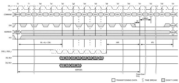
Figure 152 — Power-Down Entry after Write
