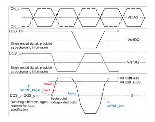
Figure 112 — Method for calculating tWPRE transitions and endpoints
