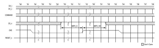
Figure 162 — CKE Transition Limitation to hold Maximum Power Saving Mode
