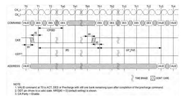
Figure 159 — Power Down Entry and Exit Timing with C/A Parity
