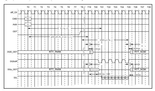
Figure 178 — Example: CL=11, PL=0; AL=CL-1=10; RL=AL+PL+CL=21; CWL=9; DODTLon=AL+CWL-2=17; DODTLoff=AL+CWL-2=17;1tCK preamble)
