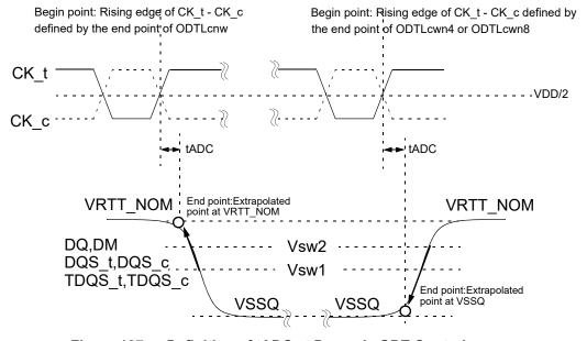
Figure 187 — Definition of tADC at Dynamic ODT Control
