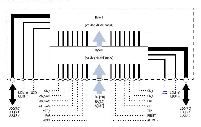
Figure 4 — Functional Block Diagram of SR x16 DDP
