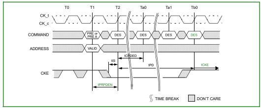
Figure 156 — Precharge/Precharge all Command to Power-Down Entry
