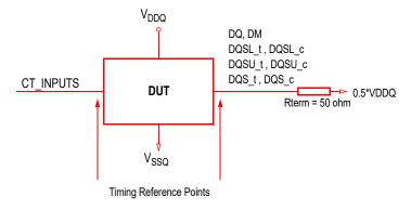
Figure 207 — Connectivity Test Mode Timing Reference Load
