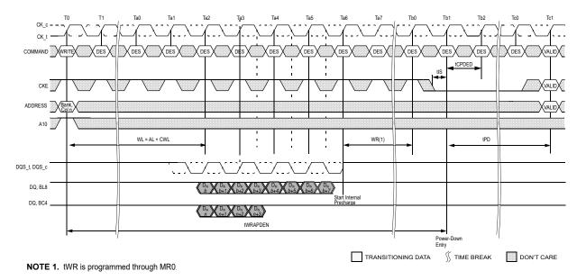
Figure 151 — Power-Down Entry After Write with Auto Precharge
