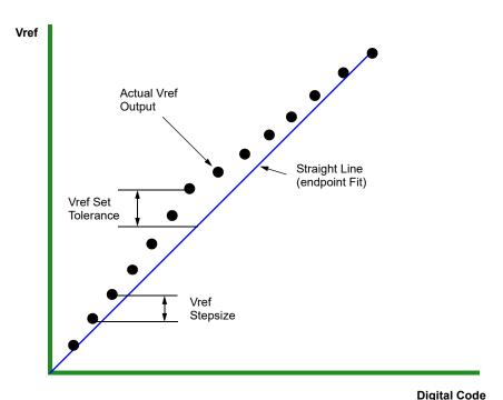
Figure 28 — Example of Vref set tolerance(max case only shown) and stepsize
