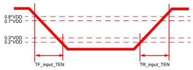
Figure 165 — TEN Input Slew Rate Definition
