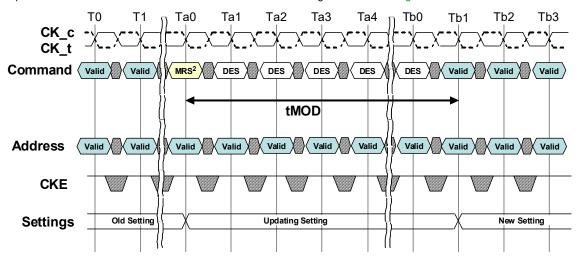
NOTE 1 This timing diagram shows CA Parity Latency mode is "Disable" case.
