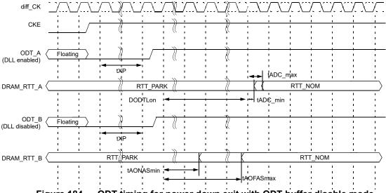
Figure 184 — ODT timing for power down exit with ODT buffer disable mode
