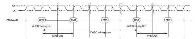
NOTE 1 The MR command used to enter VrefDQ Calibration Mode treats MR6 A[5:0] as don't care while the next subsequent MR command sets VrefDQ values in MR6 A[5:0].
