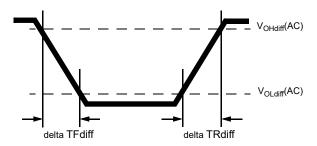
Figure 205 — Differential Output Slew Rate Definition
