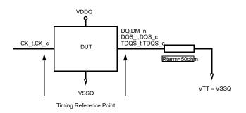
Figure 185 — ODT Timing Reference Load
