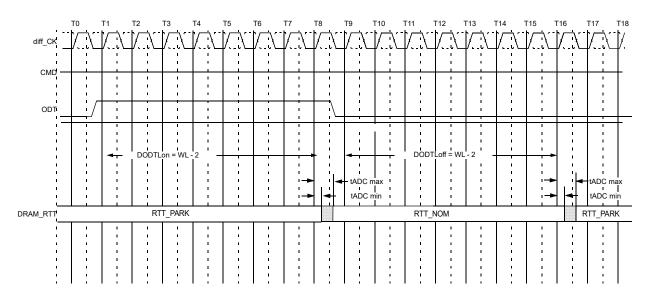
Figure 176 — Synchronous ODT Timing Example for CWL=9, AL=0, PL=0; DODTLon=WL-2=7; DODTLoff=WL-2=7
