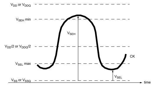
Figure 191 — Single-ended requirement for differential signals.
