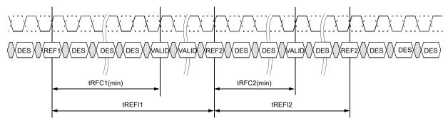
Figure 17 — On-the-fly Refresh Command Timing
